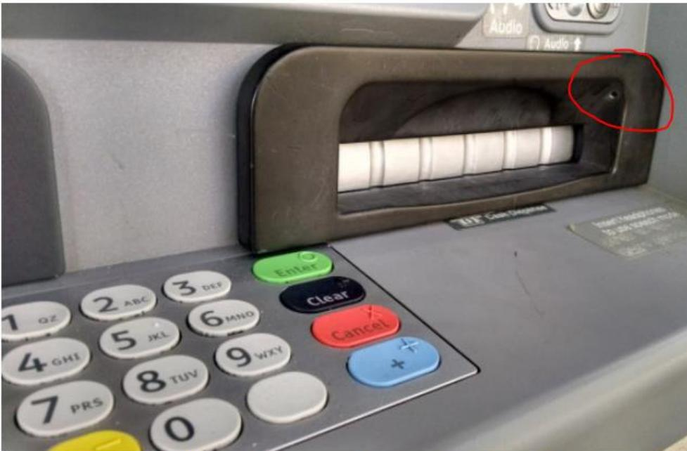
*A closeup of the tiny pinhole that allows a mini spy camera embedded in the fake cash dispenser bezel to record customers entering their PINs.*
